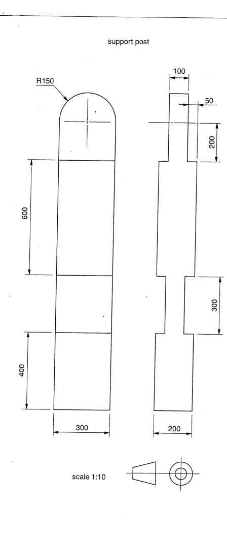
A3 A support post for a temporary barrier is drawn to a scale of 1:10 in the orthographic views given to the left.
